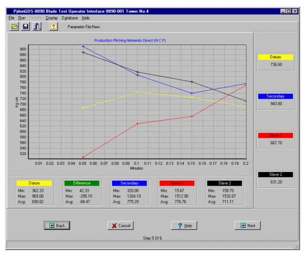
The Pylon GDS system is a general purpose, graphic display system for operator inter-action and control of intelligent plant equipment. The 8890 variant has been configured for use with fast analogue data acquisition systems, to fully automate the data collection and testing of rotor blades on balancing towers.
