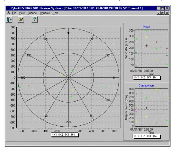
The Pylon GDS system is a general purpose, graphic display system for operator inter-action and control of intelligent plant equipment. The 8642 variant has been configured for use with vibration data collection and analysis, to fully automate the remote monitoring of major plant items such as generator sets from a central location.
