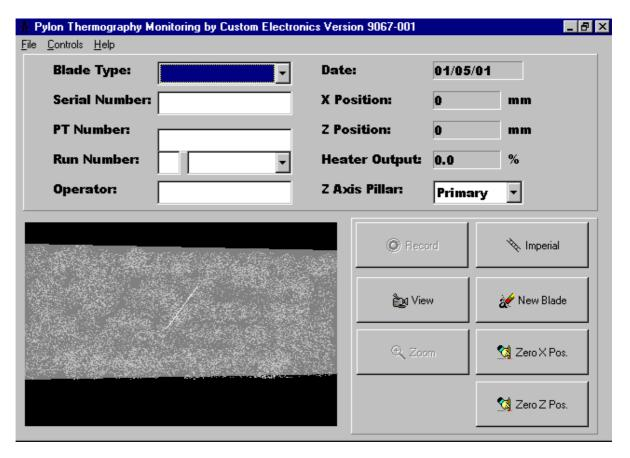
The Pylon GDS system is a general purpose, graphic display system for operator inter-action and control of intelligent plant equipment. The 9067 variant has been configured for use with composite material thermography installations, to fully automate the thermal inspection sequence of composite components from a central location.
