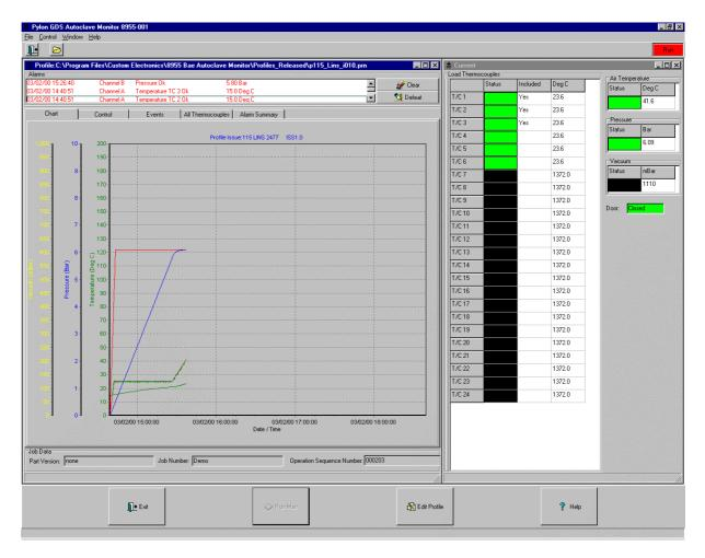
The Pylon GDS system is a general purpose, graphic display system for operator inter-action and control of intelligent plant equipment. The 8955 variant has been configured for use with composite material autoclave curing installations, to fully automate the sequence of composite component cures from a central location.
