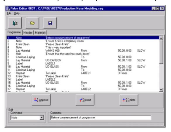
The Pylon GDS system is a general purpose, graphic display system for operator inter-action and control of intelligent plant equipment. The 8637 variant has been configured for use with composite material tape layer installations, to fully automate the laying sequence of composite components from a central location.
