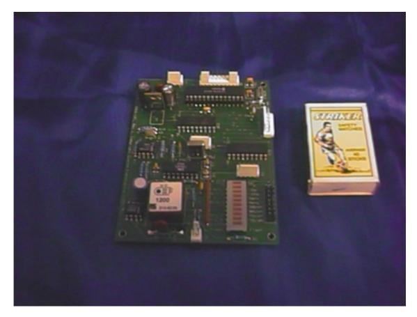
The 8926 Outstation is a general purpose, intelligent outstation designed for fast, flexible system building for mission critical control systems.
