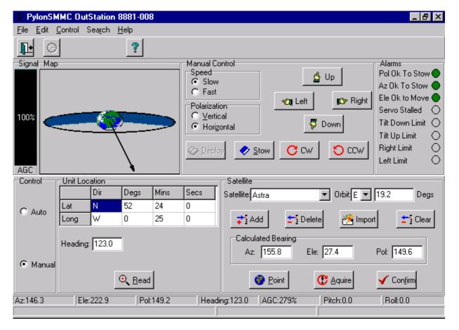
The Pylon GDS system is a general purpose, graphic display system for operator inter-action and control of intelligent plant equipment. The SMMC variant has been configured for use with satellite broadcast antenna mounts and equipment, to fully automate the remote control of truck mounted SNG Ae from a central location.
