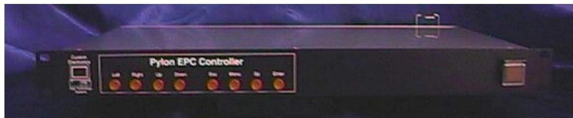
The front panel of the PylonEPC controller is contained in a 1U 19“ rackmounting format and contains a guarded, illuminated latching push button switch for mains power on/off.
