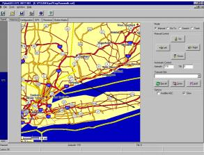
A user friendly GUI allows the user to control both steerable and horn antennae using user-configurable Maps for convenience. In normal operation the user drags the azimuth pointer on the display to the correct area of transmission. The peak search and manual GUI (and keyboard) controls can then be used for fine-tuning. During this time the audible AGC facility can be used in multimedia PC's to give an audible guide to signal changes.
