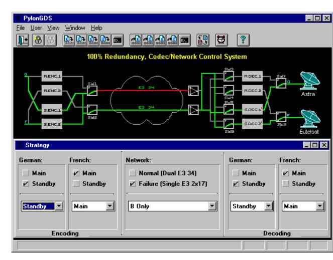
The Pylon GDS system is a general purpose, graphic display system for operator inter-action and control of intelligent plant equipment. The 8657 variant has been configured for use with codec transmission equipment, to fully automate the remote supervision and redundant control of equipment and networks from a central location.
