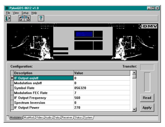
The PylonGDS system is a general purpose, graphic display system for operator interaction and control of intelligent plant equipment. The 8612 variant has been configured specifically to handle Remote Configuration of the Digi-Media Vision Ltd DSNG Codec based on Remote Control Interface Specification 10 June 1996 Draft D.
