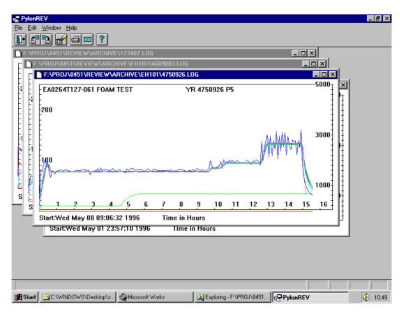
The PylonGDS system is a general purpose, graphic display system for operator interaction and control of intelligent plant equipment. The companion 8512 Review package has been produced specifically to allow the graphical review of logged data from PylonGDS systems.
