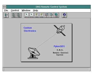
The Pylon GDS system is a general purpose, graphic display system for operator inter-action and control of intelligent plant equipment. The SNG variant has been configured for use with satellite broadcast equipment, to fully automate the remote supervision and control of SNG transmit sites from a central location.
