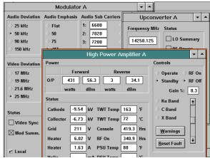
Continuous alarm monitoring is carried out by the system with the operator notified of both detail and summary alarms and also on communication failure with the remote sites.
